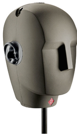
Fig. 2 Neumann KU 100 dummy head system, used for binaural recordings (Neumann)
